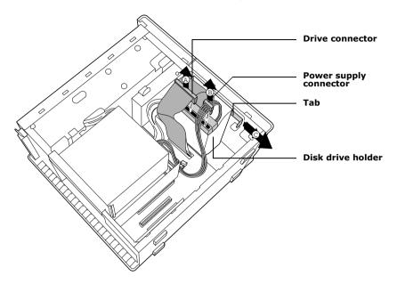
3 Disconnect the drive connector (A in diagram).
